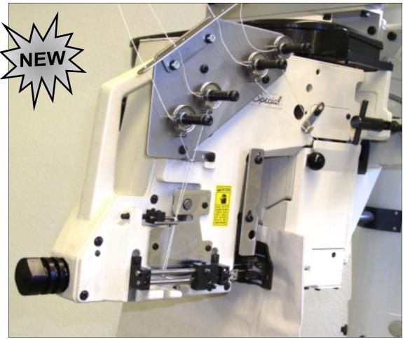
High speed and high performance two needle independent row double locked chainstitch bag closing machine for closing filled sacks and bags.
